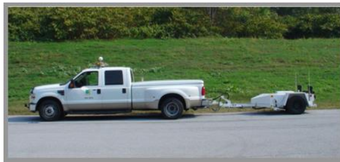
Figure 4.4 Locked-Wheel Skid Trailer
