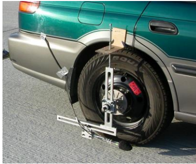
Figure 4.5 Noise Measurement Device
