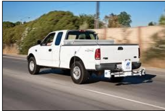
Figure 4.3 High Speed Profiler
