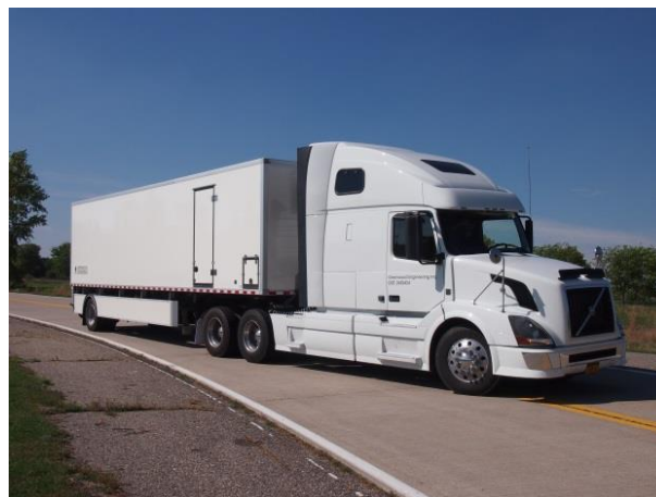
Figure 4.6 High Speed Deflectometer
